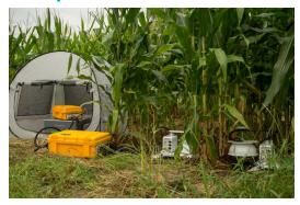
**Figure 7**. A multiplexed LI-8100A System deployed with the Picarro G2508.
