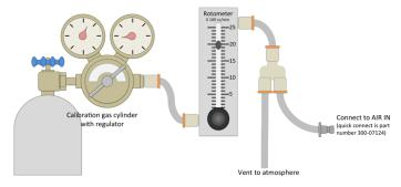
**Figure 3**. Calibration rig used to calibrate the LI-8100A at operating pressure.
