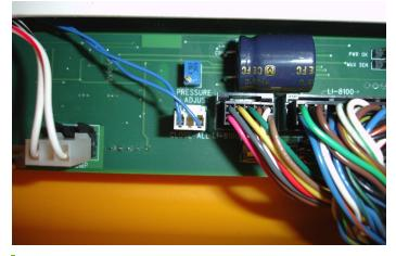
Figure 2. Pressure Adjust potentiometer.
