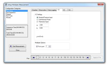
**Figure 4**. Analog input settings. For a linear voltage input select General Purpose Input and use the m and b coefficients to scale the raw voltage to meaningful engineering units: recorded value =  $mV_{in}$  + b. In multiplexed configuration use **Fix to port**: to route the analog inputs from one chamber to all the other chambers. This will ensure that the third party analyzer's data is recorded in the correct location in the data file.
